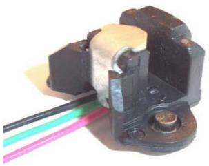
The standard length of the leads is 150mm Diameter: Ø1.4mm
